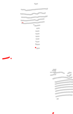
Figure 4.12.: Removal of outliers with statistical approach
